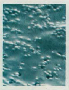
Tri-Flon Teflon® with boundary film is 20,000 times actual size, demonstrating evening-out effect Tri-Flon gives all metal surfaces it occupies. Boundary fluid displaces moisture. Teflon® particles displace microscopic space. Combination provides as smooth a non-abrasive surface as is possible to achieve.
